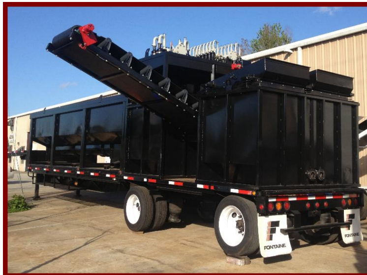
SRO60 Oilfield Wellhead Mobile Remediation Service Unit Processes 60 Tonnes Per Hour
